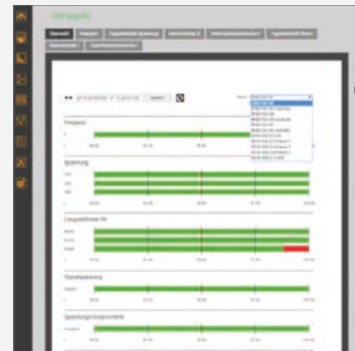
The PQ EasyReport comprises a statistical examination of power quality and can be activated freely or according to a defined standard.
